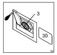
A fixed protection grill [3] prevents, as far as possible, fingers or objects from being **ACCIDENTALLY** inserted in the extraction pipe. In order to insure normal operation it is not possible to adjust the fixed grill as to prevent fingers and objects from being **VOLUNTARILY** inserted through the extraction pipe (according to Machines Directive 89/392/CEE and ensuing modifications, Appendix I, Art. 1.1.2.b, 3<sup>rd</sup> paragraph).
